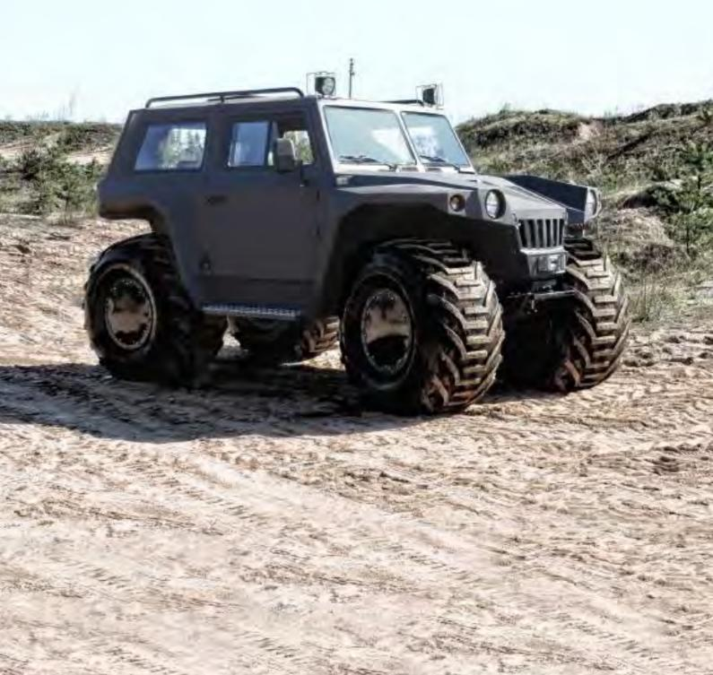
**All-terrain vehicle BME-1015** - is an all-wheel drive, multi purpose vehicle, designed for delivery of cargo and equipment, human transportation, as well as for repairing, emergency and patrol work in different road conditions, mainly for natural soil roads and cross-country, for the soils with low bearing capacity including snow virgin soils, sands, tabel soils of tundra as well as swamps.
